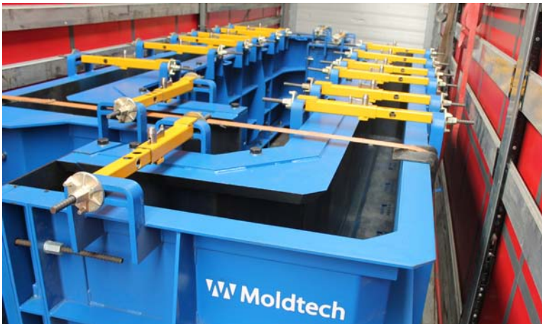
Detail of upper fastening bars
