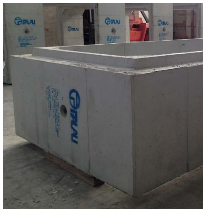
Base prepared to leave the female part of the joint of the joint
