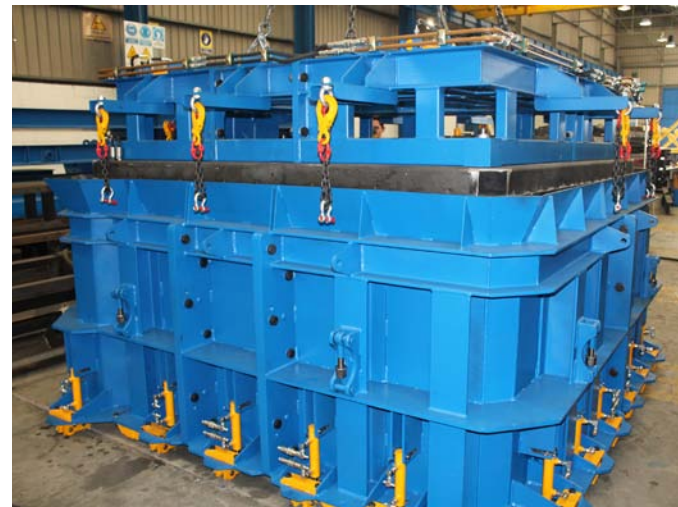
Press for making male part of dovetailing joint
