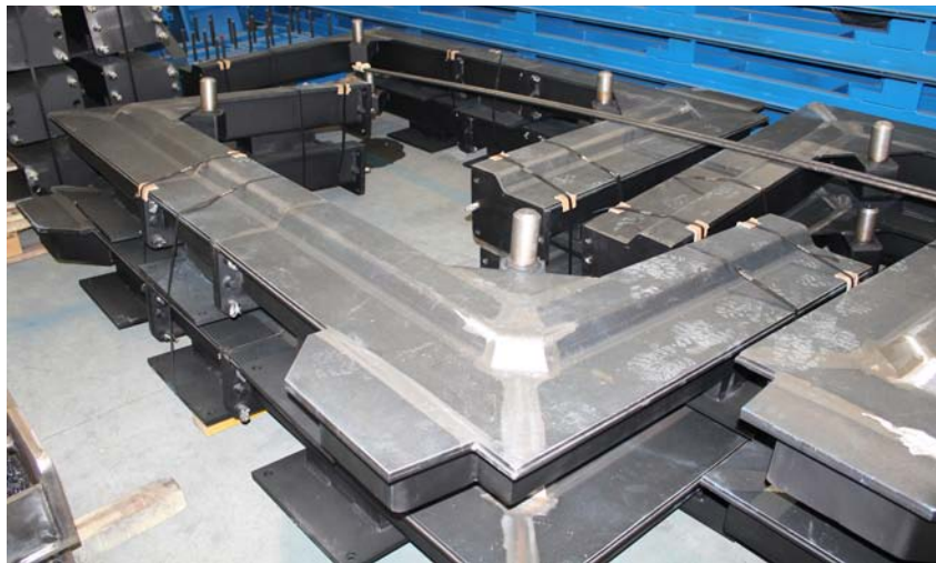
Sets of bases prepared for female part dovetailing in the piece
