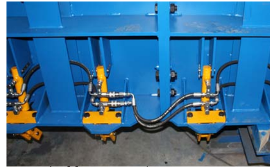
Detail of fastening clamps
