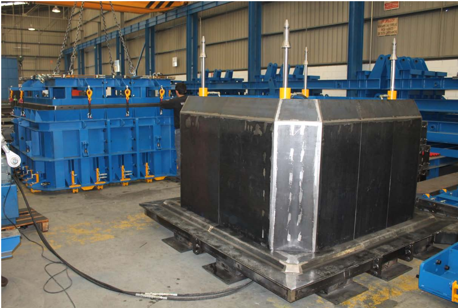
Detail of inner mould with hydraulic cylinders for upper press activation
