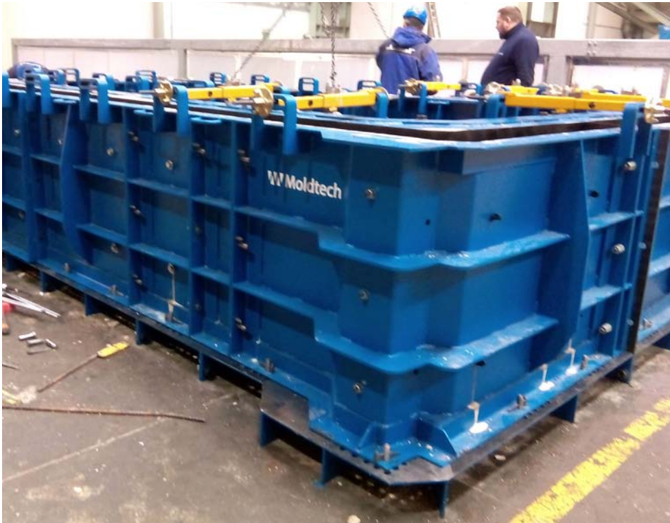
Detail of mould for piece with optional corbel
