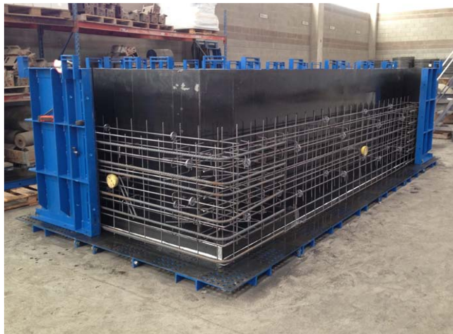
Base prepared to leave the female part of the joint of the joint
